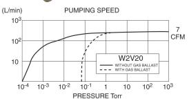
The FluidX W2V20 rotary vane vacuum pump features a rugged, two-stage, air-cooled design and is capable of pumping speeds of 7 cfm and producing an ultimate vacuum of  $10^{-3}$  Torr. Lightweight, quiet, and compact, the W2V20 features an anti-suckback and gas ballast valve, quick disconnect ISO/KF fittings, and is ideal for a variety of applications.
