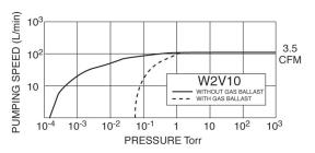
The FluidX W2V10 rotary vane vacuum pump features a rugged, two-stage, air-cooled design and is capable of pumping speeds of 3.5 cfm and producing an ultimate vacuum of 10<sup>-3</sup> Torr. Lightweight, quiet, and compact, the W2V10 features an anti-suckback and gas ballast valve, quick disconnect ISO/KF fittings, and is ideal for a variety of applications.
